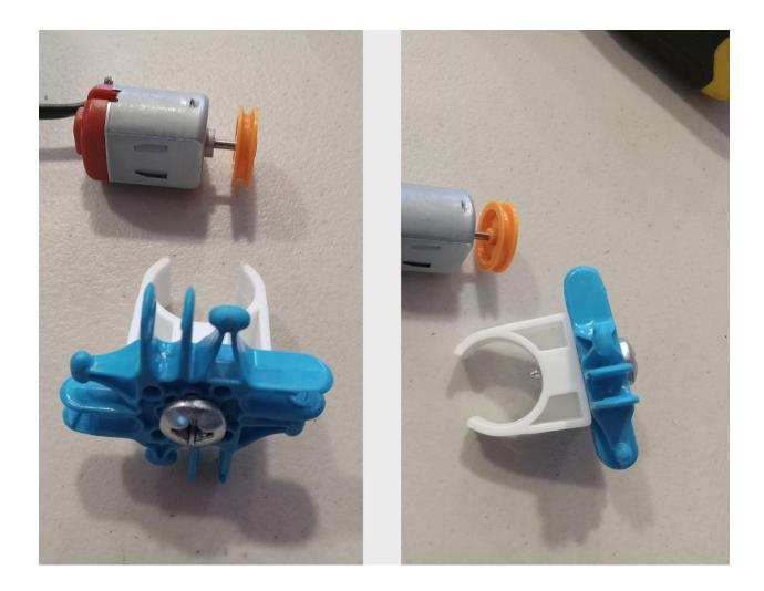
The motor is clipped into the mount. The wires must go toward the clip for the motor to fit into a four Blox square. If you use the  $\frac{3}{4}$ " screw, you must watch for the tip sticking through the mount. Make sure it is mounted like the photo
